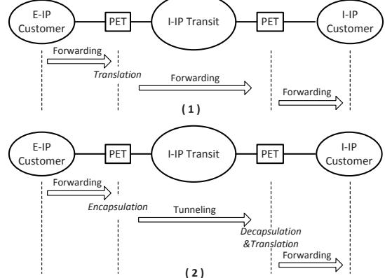
Fig. 4. PET communication model design for E-IP=>I-IP=>I-IP
