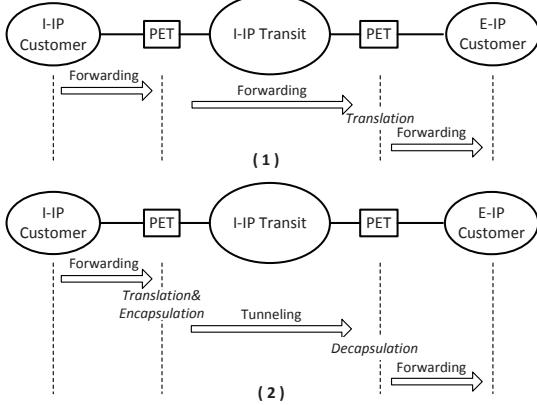
Fig. 5. PET communication model design for I-IP=>I-IP=>E-IP
