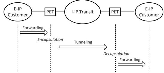
Fig. 3. PET communication model design for E-IP=>I-IP=>E-IP
