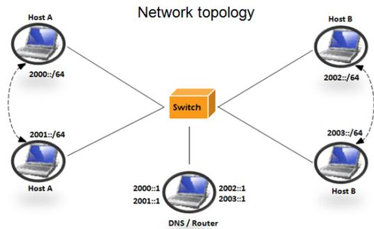
Figure 2: Testbed topology
